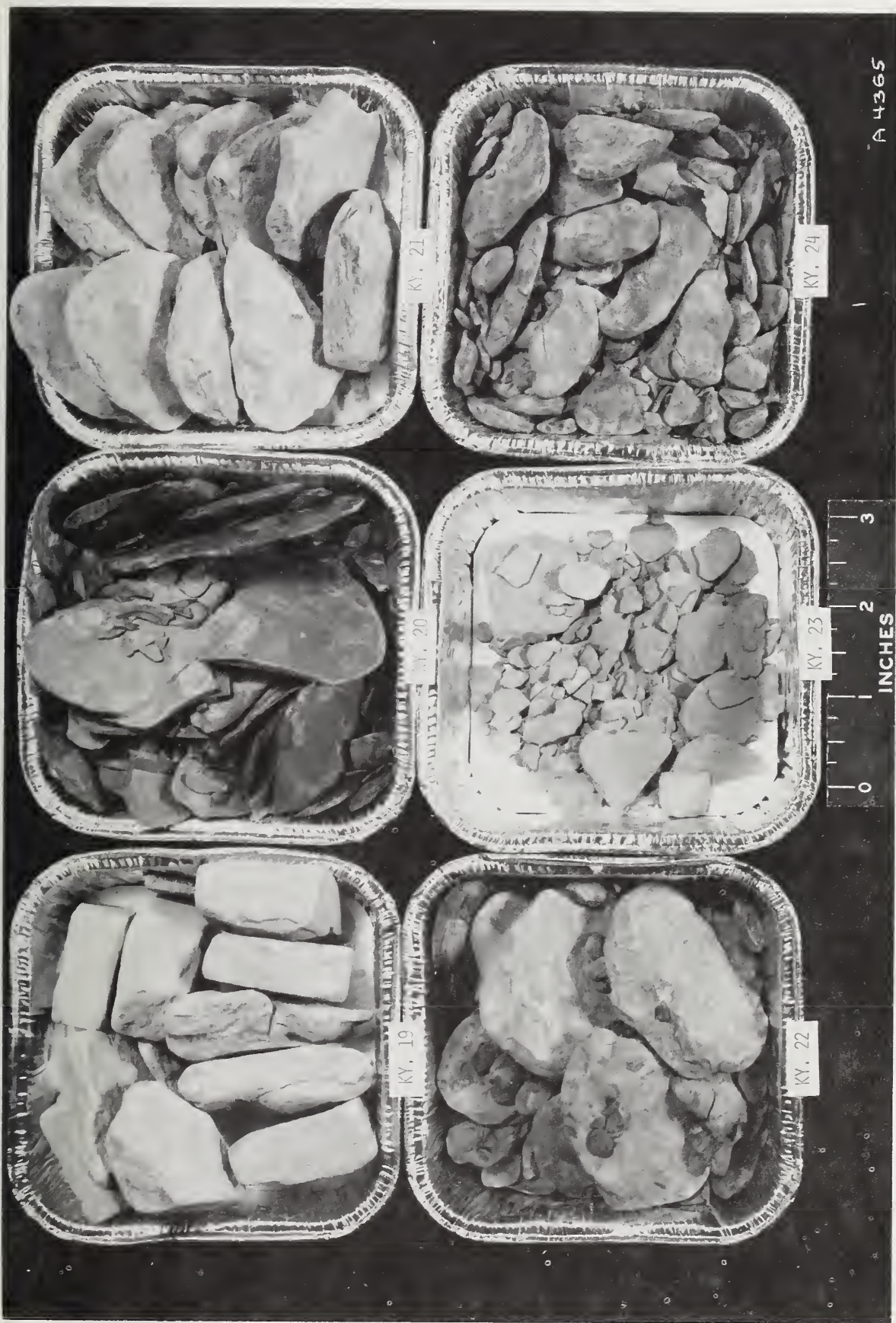
Figure 40. Material remaining after slake-durability testing, KY 19-KY 24.
